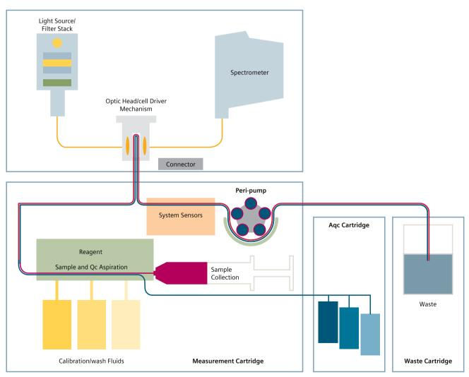
Figure 5. System fluidics schematic: Patient and QC flow paths are the same from sample entry to waste.
