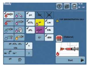
Figure 2. RAPIDPoint 500 system automatically reports acceptable QC results for multiple analytes and indicates when QC and calibration routines are unacceptable.
