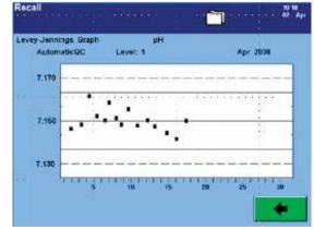
Figure 4. Levey-Jennings graph showing Level 1 AQC results for pH over time on a RAPIDLab 1200 system.
