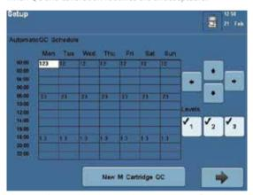
Figure 3. Siemens blood gas analyzers can be configured to meet user-defined QC schedules. Fully customizable QC schedules include selecting the day, time interval and level of QC to be run.
